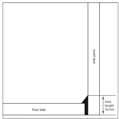
For correct dimensioning of the adhesion joint we advise a minimum joint width of 2 mm, depending on the strength of the glass. At a strength of 8 mm we advise adhesion joints with a width of 2 - 3 mm and at a strength of 12 to 15 mm a width of 3 - 4 mm.
